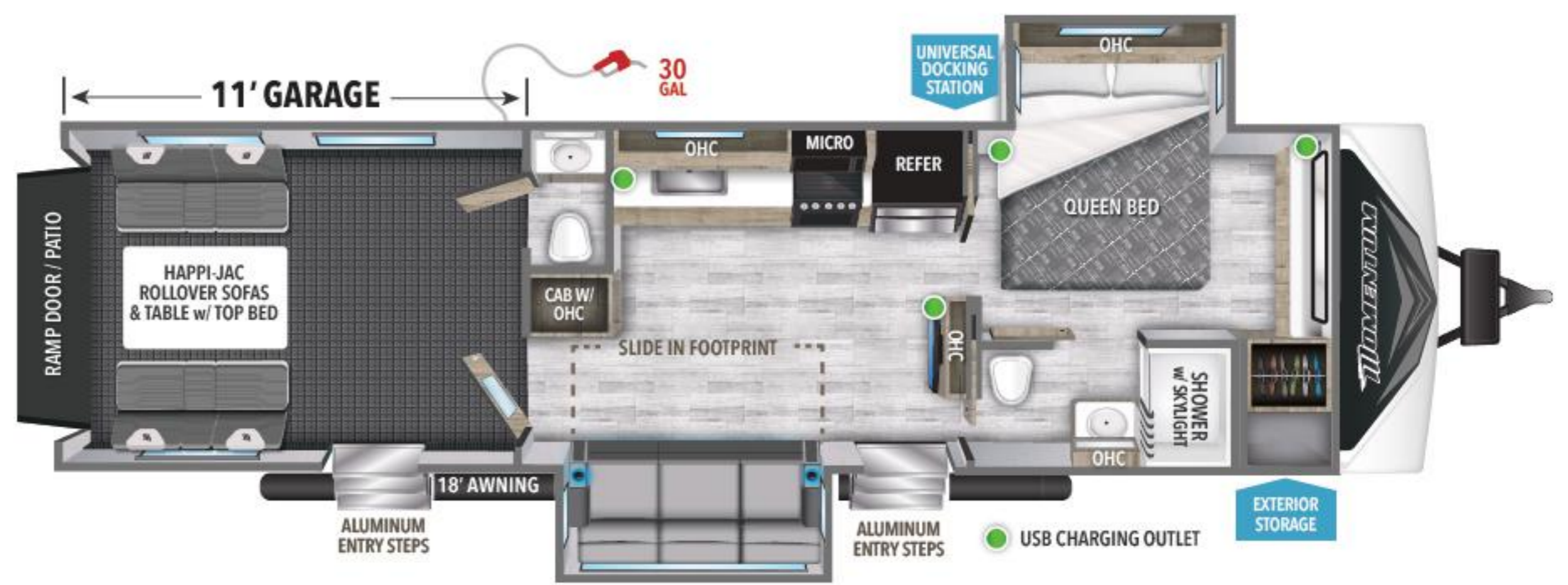
29G 11' GARAGE UVW' EMPTY HITCH' GVWR LENGTH' HEIGHT CAPACITY 8,700 1,500 13,000 33' 11" 12' 4" 96 37 39 37* *1/2 BATH DOUBLES AS BLACK/GREY
